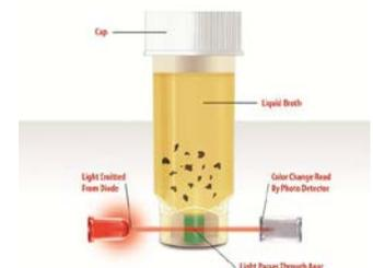
metabolic processes occur. Color changes in the vial's agar plug are monitored every six minutes and expressed as optical units. These changes are recorded in the computer, thus enhancing traceability. The more organisms there are in the sample, the faster the agar plug changes color and the faster Soleris records detection.
