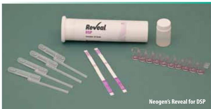
Reveal® for DSP detects the DSP-causing okadaic acid group of toxins that can occur naturally in shellfish. The assay is a highly sensitive dipstick test designed for the qualitative screening of shellfish for okadaic acid, with the visual cut-off value for a positive result set at 160 ppb.
