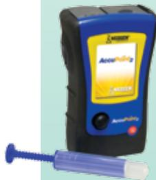
AccuPoint® 2 Sanitation Monitoring System can measure the ATP, the energy carrier for all living cells, collected from surfaces inside poultry houses. AccuPoint works by measuring the light created when ATP contacts a reagent in the system's unique sampling devices. The higher the levels of microorganisms in a surface sample, the more ATP, and the more light produced.
