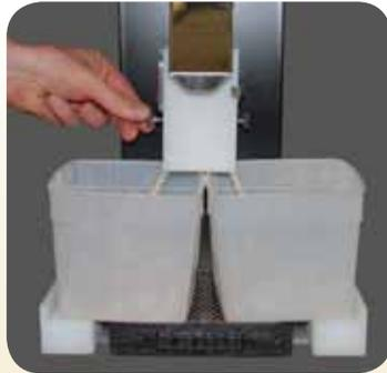
Neogen's new sample divider (Neogen item #9517) is an easy-to-install attachment for the grinder that equally separates two representative samples as you grind.
