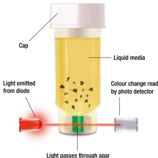
“ The Soleris method is easy to implement: 5 mL are inoculated into a ready-to-use broth. The optical reading and interpretation of the results are performed automatically (without visual assessment). The results obtained are plotted, and the growth curve allows additional information to be obtained for the interpretation of results. ”
